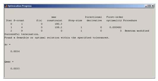
The **Optimization Progress** window shows the new optimized parameter values of  $0.0036~\text{m}^2$  for the cross-sectional area of the piston, and  $0.0033~\text{m}^3/\text{s}$  for the pump flow rate. These values are also changed within the MATLAB workspace.
